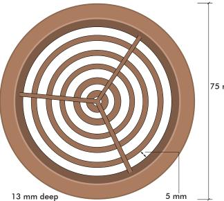
Circular Soffit Vents are easy to install, providing eaves ventilation through the soffit for new build or re-roofing.
